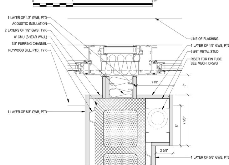
10 WINDOW PLAN DETAIL @ PARTITION WALL (SHEAR WALL)
